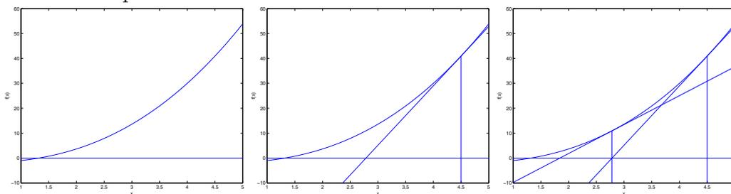
In the leftmost figure, we see the function  $f$  plotted along with the line  $y = 0$ . We’re trying to find  $\theta$  so that  $f(\theta) = 0$ ; the value of  $\theta$  that achieves this is about 1.3. Suppose we initialized the algorithm with  $\theta = 4.5$ . Newton’s method then fits a straight line tangent to  $f$  at  $\theta = 4.5$ , and solves for the where that line evaluates to 0. (Middle figure.) This give us the next guess
